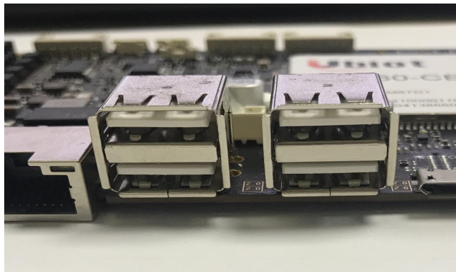
Figure 5 : USB HOST interface
